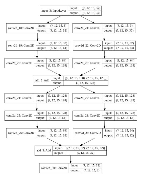
Figure 4.4.: Best performing architecture for a deep convolutional autoencoder with separate horizontal and vertical convolutions that are added in the latent space
